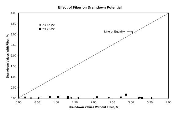
Figure 1: Effect Of Fiber on Draindown Potential (10)
