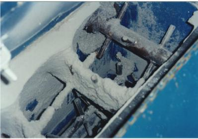
Figure 6: Fiber Pugmill-Type Dispersion System
